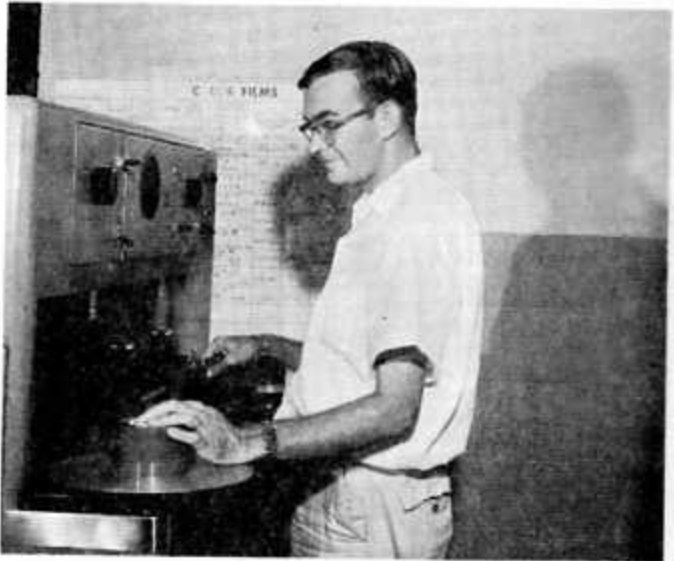
Photographic Standards technician J. J. Ondera tests film samples on a sensitometer.
