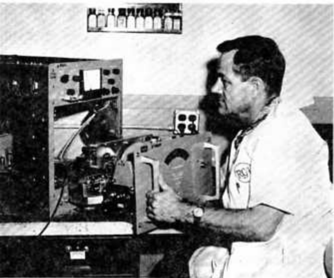
Electronics Technician Sherman Bell (Cape Canaveral TERC) trouble-shoots a plug-in microwave receiver unit.
