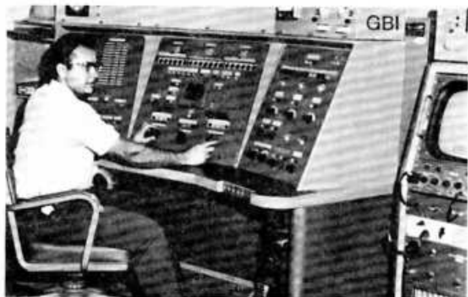
MTP's Pete Bray at the FPS-16 console, standing by to complete a radar check-out prior to a test.
