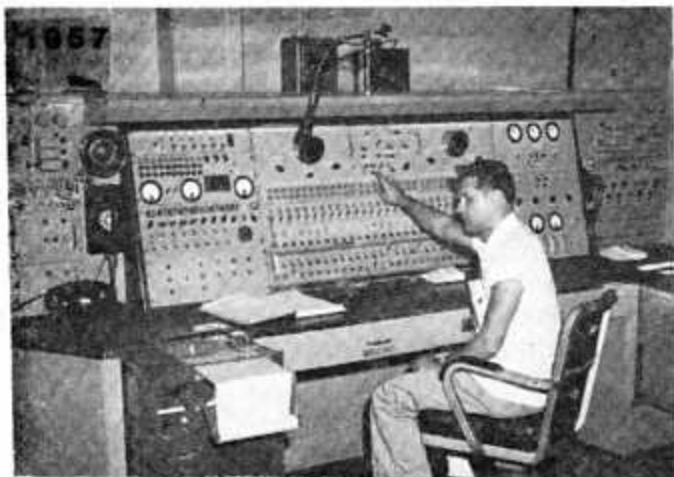
1957 Cape Canaveral Timing is synchronized with signals transmitted by WWV. Leader A. A. Terek is shown at the Central Timing Distribution Console as he prepares to synchronize the time base generator.
