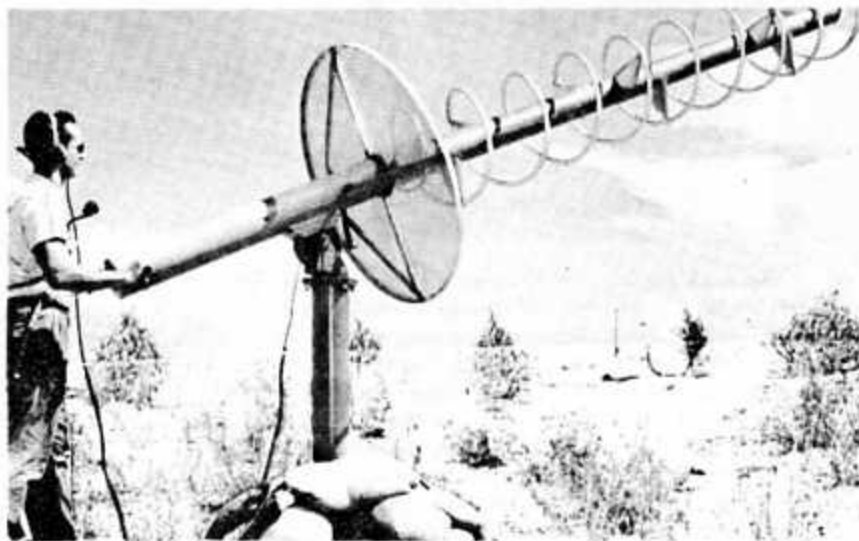
COMPLEX TELEMETRY ANTENNA receives FM signals from the missile.
