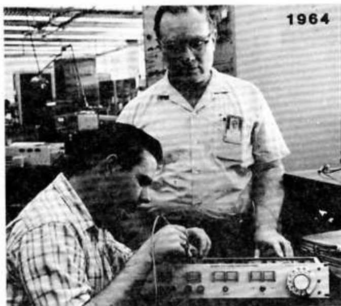
MTP's electronic shops are also constructing some of the equipment that will be used on Gemini. Here technician M. D. Hernandez assembles a Gemini communications switching panel. Looking on is Al Waits, who designed the device, of Communications Engineering.
